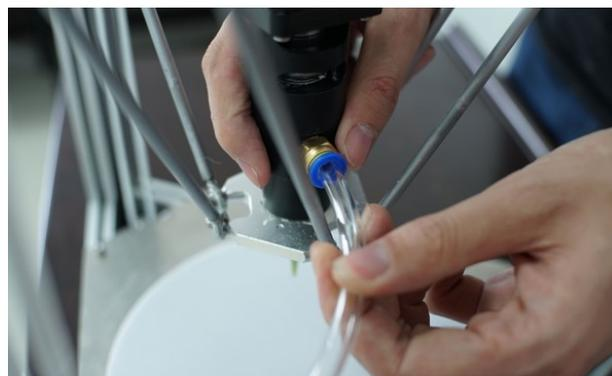
a) Screw the barrel into the push rod motor, remember to match the thread and align it. Do not twist the tooth and screw it. Before screwing, use the water to wet the tail of the barrel for easy screwing.
